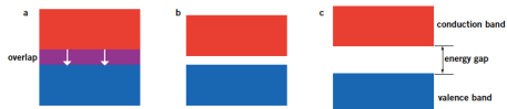
Figure 10.1.4 Energy band diagrams for (a) a conductor, (b) a semiconductor and (c) an insulator
